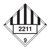
According to SP 965 it is required to mark cargo transport units with a warning mark including the words "CAUTION – MAY CONTAIN FLAMMABLE VAPOUR" which should be fixed to the doors of the container.
