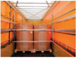
Picture 3: Examples for different load securing systems using form-lock securing
